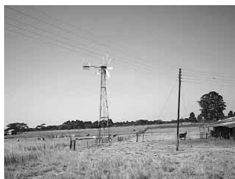
Figure 6.2 Multi-blade low speed wind pump used in Zimbabwe
